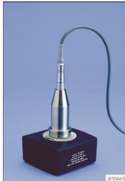
Fig. 6 Sensitivity calibration at 1 kHz using Sound Level Calibrator Type 4231
